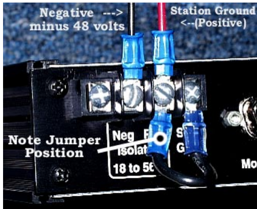
Figure 4. POSITIVE GROUND SYSTEM
