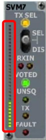
**Figure 1-10. Site Voter Module Signal Quality Level Bar Graph Display**
