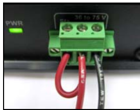
Figure 3 . Positive Ground Jumper Power Input Example
